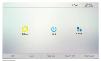
Reboot: Means reboot TS but not whole machine. Should notice that, Reboot won't automatically save parameters. Need to click "Save" button first.
