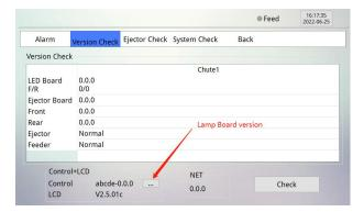
For those MS and KX model (equip with new lamp control board), click "..." will show the Lamp board version.
