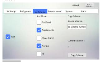
Sort Inject: For color sort arith use. Usually we disable this function. If this option is enabled, machine will reject any speckled or non-compliant material.
