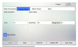
Shape first (Eject delay): We separate Color sort and Shape sort Eject Delay time for better performance. When use shape arith, this value should be set according to material and machine model.
